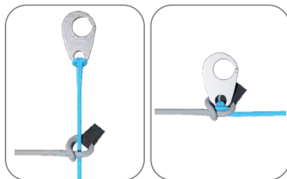
Diagram 2. Speed-bar connection by means of kite loop (without Brummel hook). The blue line is from the harness, and the gray from the riser.
