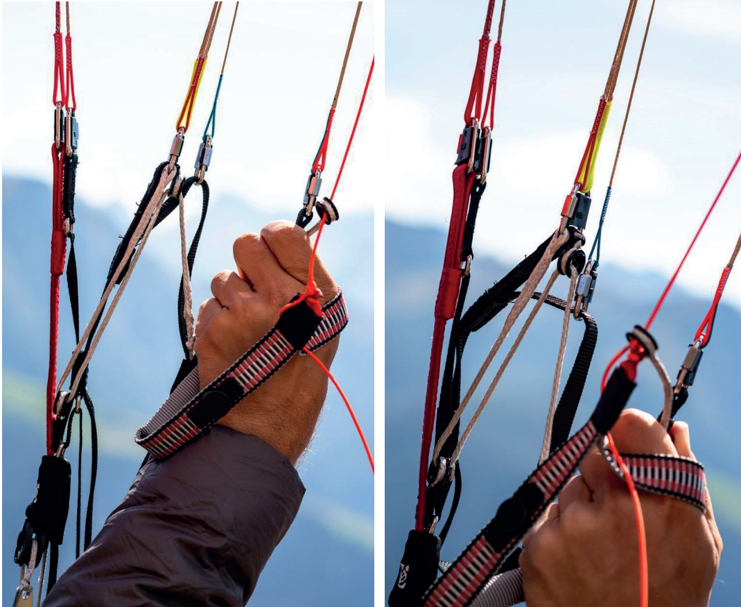
Figure: How to grab and pull the Camino smart riser
