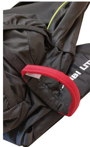
Position the handle in its folding sleeve. It may not protrude from the harness.
