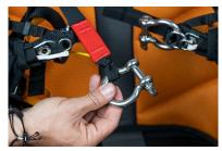
The BASE parachute is folded into the freebag and kept/stored in the rear container. The BASE deployment bag is connected by means of a strap to the right shackle, so that with the activation of the 3 ring release, the BASE freebag remains tied to the paraglider, which acts as an extractor for the BASE parachute.
