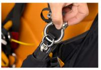
Once the harness has dried, remember to carefully recheck and lubricate all metal parts to avoid rust or deterioration.
