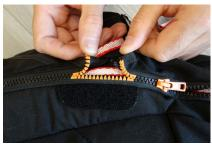
After having connected the reserve to the harness with one of the previously described systems. Insert the parachute with the lines into the harness container, taking care to place the reserve's lines towards the bottom of the harness to facilitate opening.
