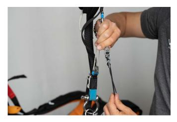
When the base handle is tensioned and the 3-ring release system is operated, the metal pin of the straight release cord will slide out of the OR releasing the speed cord and releasing the glider.
