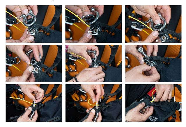
Tensioning of the release handle causes the three-ring system to open and quickly release the shackles (where the glider is attached) from the harness, causing the BASE to open.
