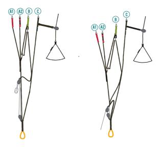
The length of the accelerator is adjusted to the left and right of the foot pedal so that when your leg is fully extended, then the acceleration is at maximum – both rollers are touching.
