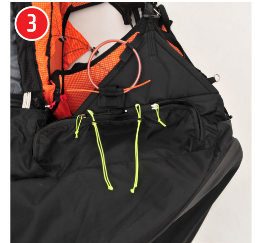
4 Pass anchor loops through outer cover eyelets
