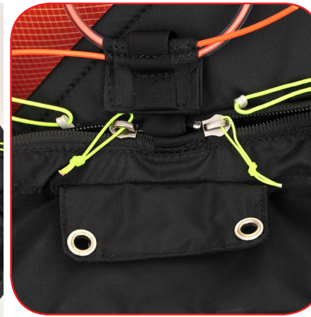
3 Make sure the rescue handle is in the middle
