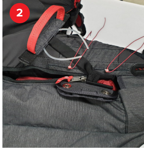
2 Make sure all lines are neatly on the bottom of the container, move zipper to the shown position and pass the parachord through the closing loops
