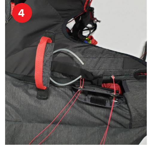
4 Use paracord to pull the closure loops through the secondary loops and metal eyelets
