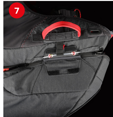
Secure the handle wire in the housing left and right as shown and slowly remove paracords
