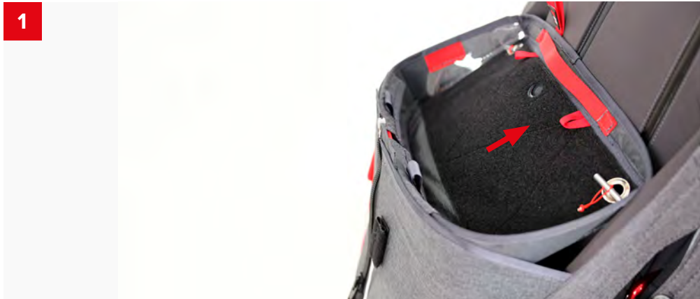
1 Keep the flight deck in a high angle position before take off, the stick lines will pull the flight deck to the right flying position once airborne.
