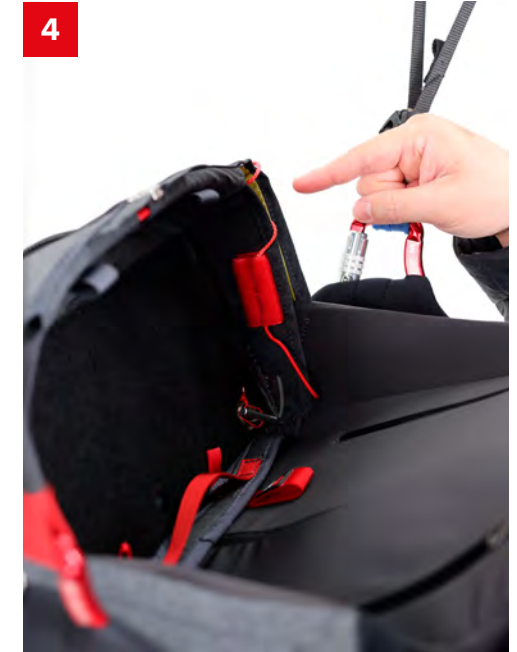
4 Store the extra line in the dedicated pocket and stick the velcro on the side of the flight deck
