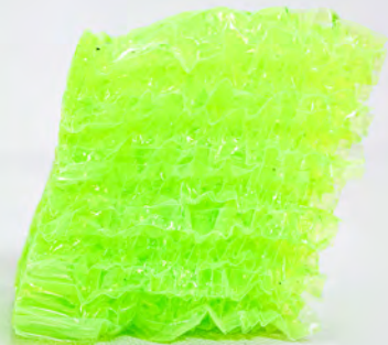
Damaged cell (Needs to be replaced)
