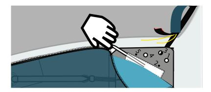
Using the safety pin, push the handle's short cable through the white lanyard loop and through grommet #1, then the end of the cable in hole #2.
