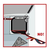
Fasten the handle on the side panel by sliding the tong in the receiving slot, and then placing it on the Velcro®.
