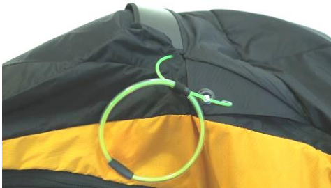
Fig. 37 feeding the long pin into the rescue compartment
