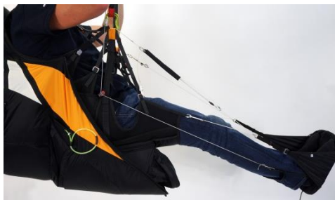
Fig. 51 Adjusting speed bag length
