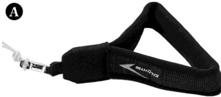
Multigrip brake handle on delivery with both stiffeners
