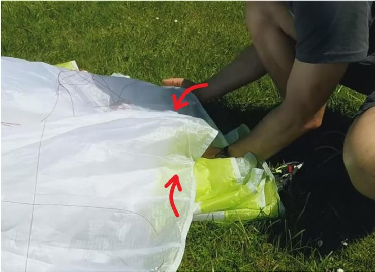
6. By using the standard „AirPack“, the whole glider will be put into the inner-bag first, then closed, and then folded to the required length and fixed with the straps.
