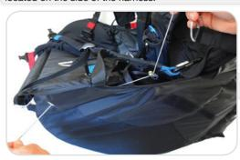
Then pass the line on the inside of the outer panel and out through the eyelet.
