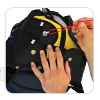
Close the clover leaf flaps in numerical order using a suitable piece of magic string or plastic threaded through the white loop on flap no.1. Pull the loop through all of the numbered flaps.
