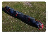
**Step 9**. Turn the Concerto on its side and make the first fold just after the LE reinforcements. Do not fold the plastic reinforcements, use 2 folds around the LE.
