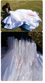
**Step 3.** Lay wing on its side and Strap LE...Note the glider is NOT folded in half; it is folded with a complete concertina from tip to tip. It is really important to not stress the middle cell or bend the plastic too tightly.
