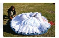
Step 2. Group the Leading Edge (LE) reinforcements with the A tabs aligned. Make sure the plastic reinforcements lay side by side.
