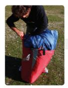
**Step 6.** Fold the wing with 3 or 4 folds whilst being careful to not crush the LE.
