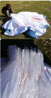
**Step 4.** Group together the middle/trailing edge of the wing by sorting the folds near the B, C and D tabs.
