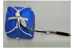
3. Insert the inner container so that the suspension lines point outwards / upwards. Let the handle run out between the container flaps 3 and 4.
