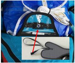
Insert the handle cover under the container flap 4. Place the handle cover over the container flap 3 and under the container flap 5.
