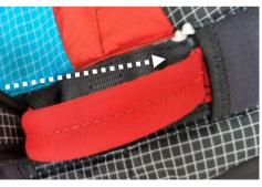
After each pack, a test activation must be carried out and checked to ensure that the opening force is not more than 7 daN.
