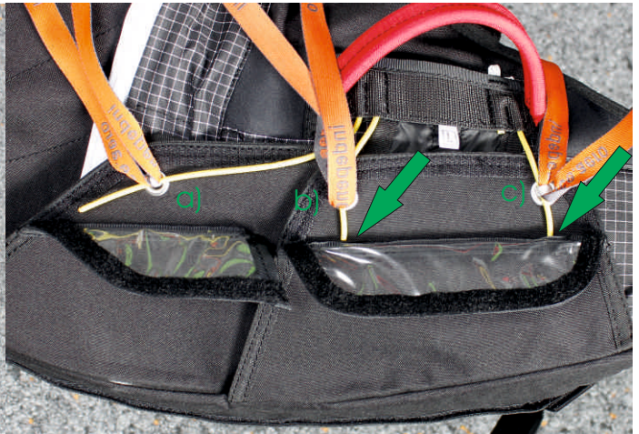
8. Insert the excess cable from b) and c) into the slot in the container flap.
