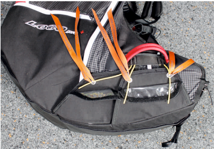
7. Close the front container flap and secure it with the cables.
