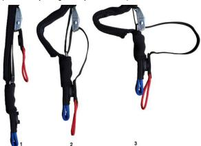
Position 1 is to be used if the passenger is significantly taller than the pilot. The difference is 6 cm In position 2, the pilot and passenger are at the same height
