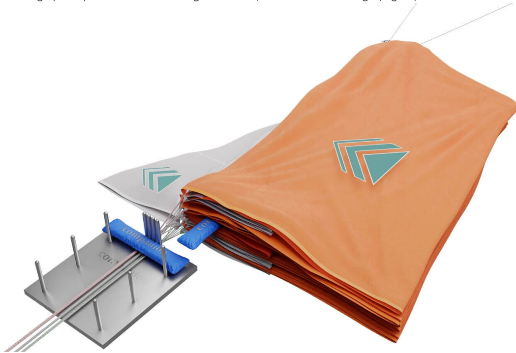
Fig. 30 Prepared side fixed in place; left side now on top
