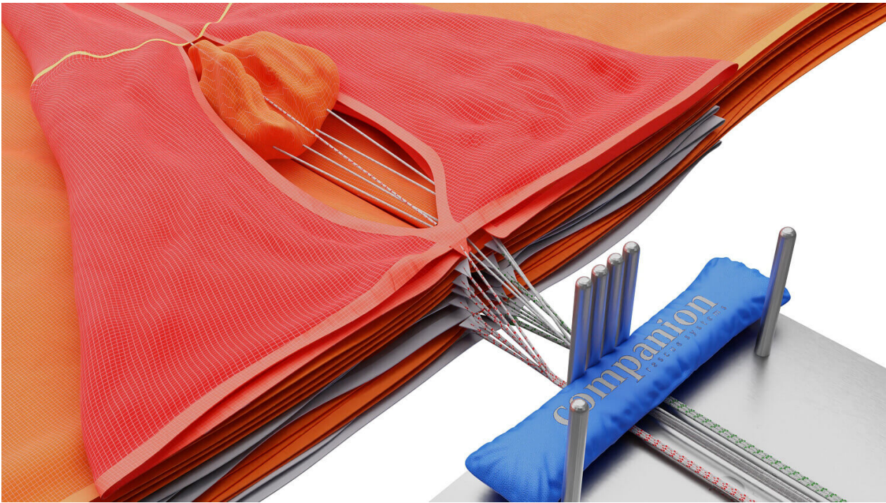
Fig. 31 Middle of the canopy bulging out
