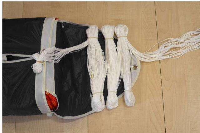
The suspension lines are sorted in three bundles, which are fixed by rubbers.
