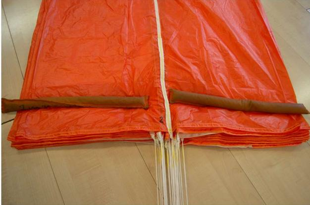
Put a packing weight for fixation on the last panel and then all the panel from the right side can be shifted to the that side.
