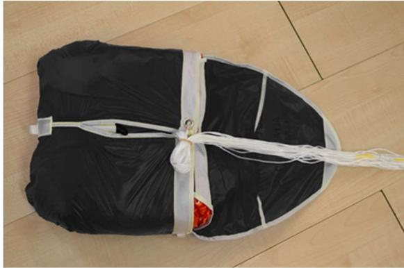
Close both sides of the inner container and the top pocket with the rubber, which you fix with one loop of all the suspension lines.
