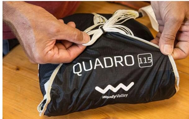
With the rest of the suspension lines you finalize the closing of the inner container by pulling the suspension lines through the black rubber loop. Don't make the closing loop too big.
