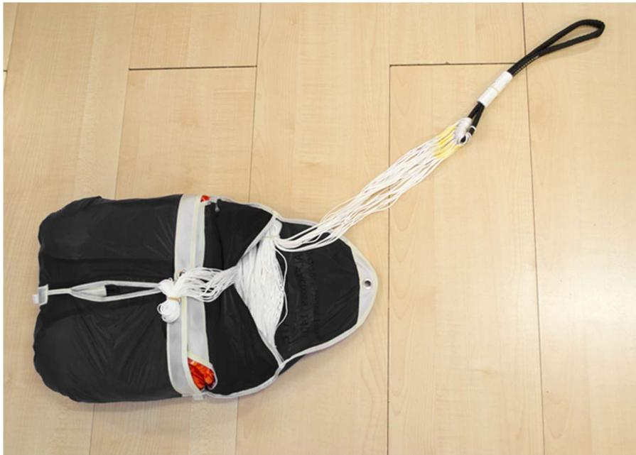
Use the last 20 cm of the suspension lines for the final closing of the inner container with the black rubber.
