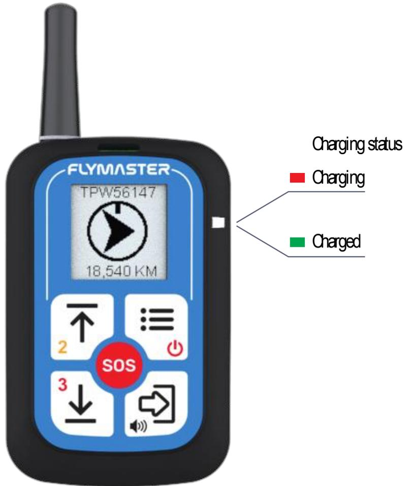
Note: Charging the instrument with high ambient temperatures should be avoided. Such action can cause the battery to overheat and affect the battery health.
