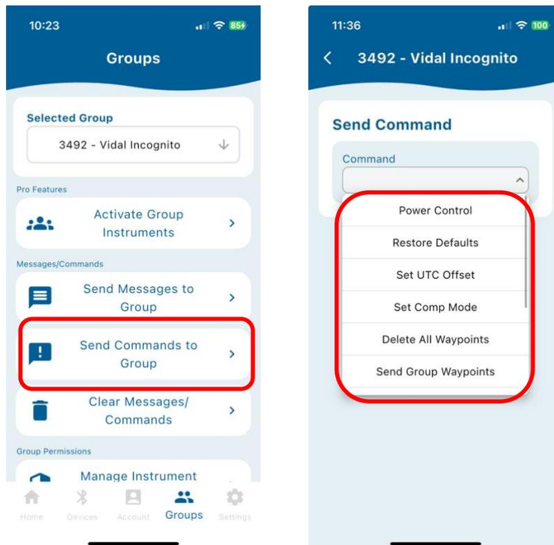
The **"Send Commands to Group"** tool allows you to send **remote commands** to control the group devices.
