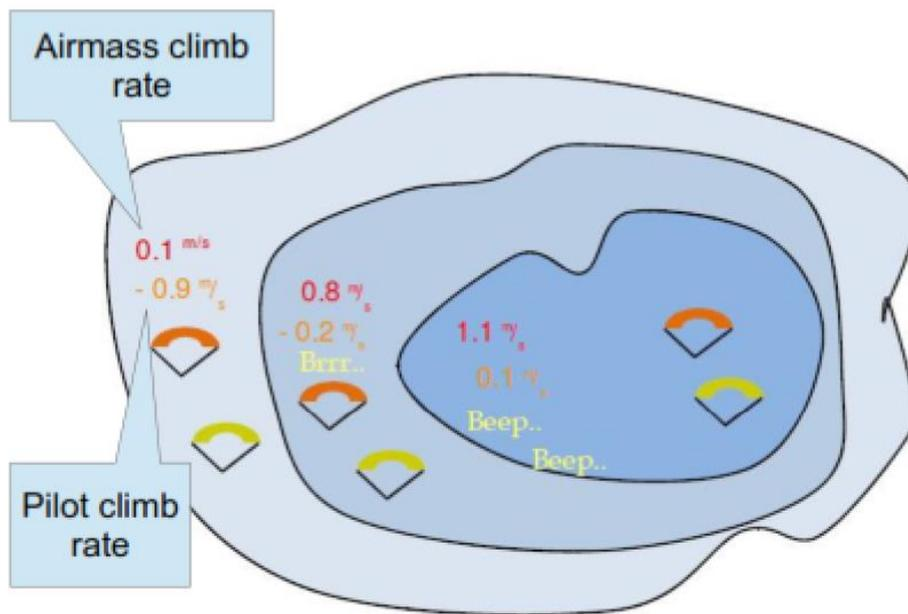
**Cadence** - When a rate of climb is higher than that specified by the Climb threshold the LIVE ONE creates a beeping sound. The rate (cadence) of the beeps increases as the climb rate increases. This increase in rate is not linear. The cadence parameter specifies which cadence curve should be used. Current there are 2 possibilities represented in the graph of Figure below.
