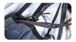
For the third attachment point, guide the horizontal attachment loop around the leg straps or the get-up system of the harness so that the front container cannot tip upwards in case of deployment.
