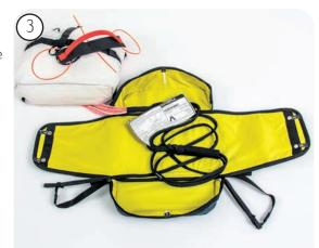
**4.** Guide the V-line to the left and right of the cover flap (with velco on top) and make sure that you have enough V-line from the front container depending on the type of assembly (main carabiner or shoulder harness mount).
