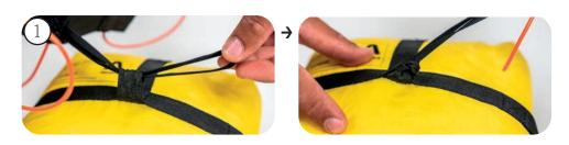
2. Now you can connect the V-lines of the EXIT with the lanyard of your reserve chute. To connect the reserve chute to the V-line, you must use a screw shackle with at least 2400 daN strength. The lines have to be connected on both sides of the screw shackle and must be secured with rubber bands (option A).
