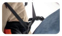
All three attachment points offer the possibility to adjust the length of the attachment. Make sure that the fasteners are neither loose in flight nor take up the main tension of the harness.
