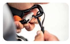
When using this method make sure that the speed bar connecting line is always routed between the harness and the V-line
