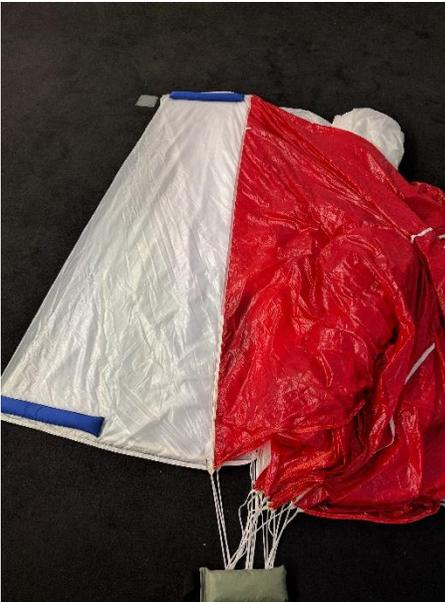
5. Arrange the other panels, always pull out the upper part as far as the panels form and they will form rectangle. Repeat with each panel till you reach the next panel with valve.
