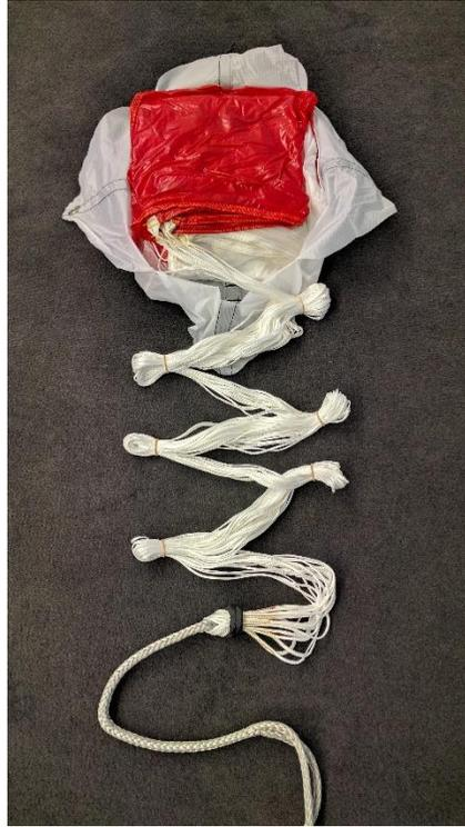
19. Hank the lines (3x3 as above) in a figure-8 format. Do not bundle the last 50cm.
