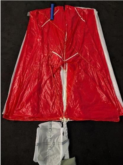
12. Fold  $\frac{1}{2}$  of the right and left sides into the center of the canopy (see picture). The width should match the width of the inner-container.
