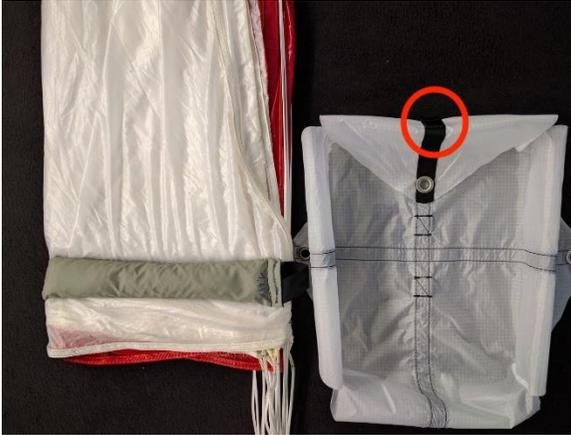
14. Place the rescue container next to the canopy, make sure that the handle attachment pointing at top of canopy!
