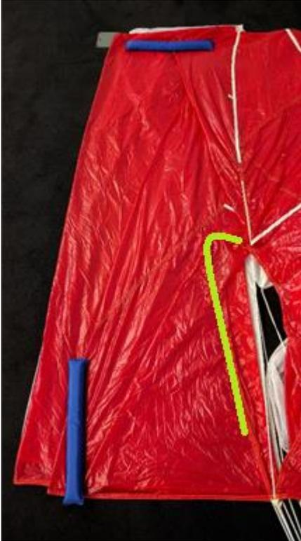
6. Arrange the panel with valve, fold the valve like shown on picture.
