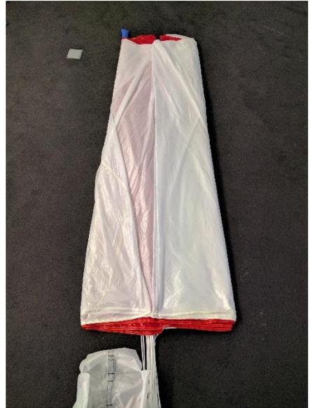
13. Fold the right part of the canopy on top of the left part. Lines and valves will be on the right side now. Width of the canopy and the inner-container should be the same now.
