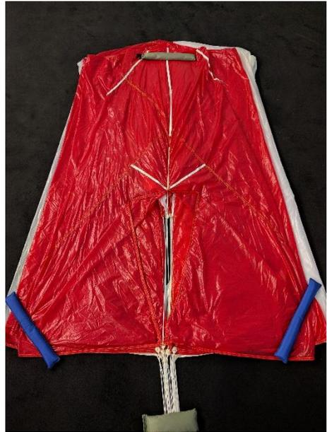
10. Pull out panel 1 on the floor. Arrange the other panels, utilizing the same process as you have for the left side until you reach panel no 9 (with valve) which will now be situated on top.
