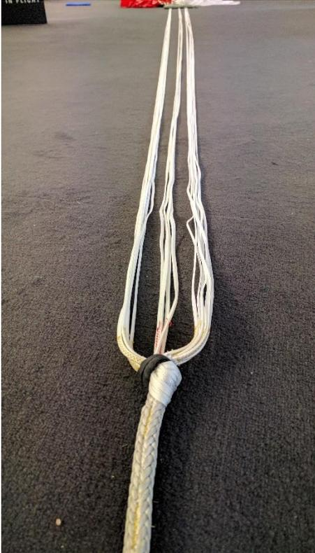
1. Lay the lines straight, separate the centre lines from the base lines
