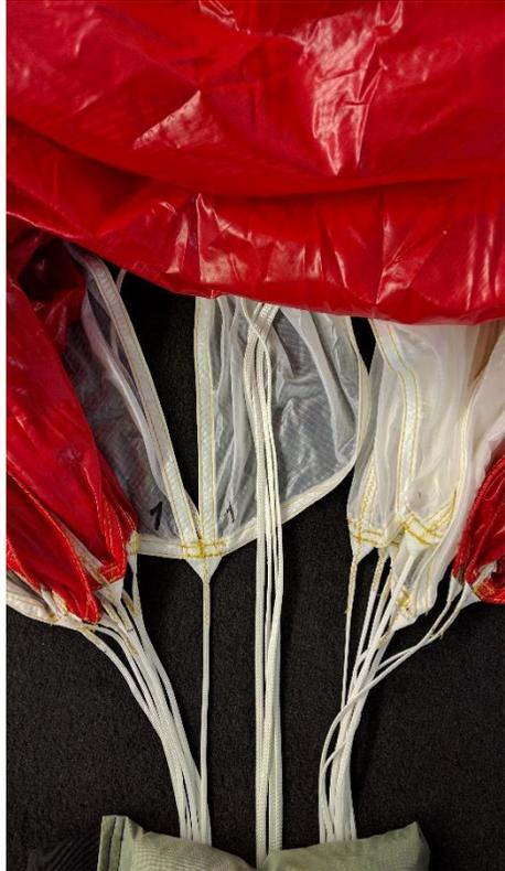
2. Panel 1 (panel with valve) must be the bottom panel.
