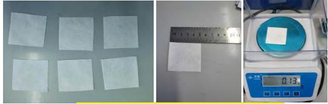
Item #4 : critical material ( filter blown fabric) checking
