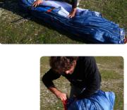
**Step 6.** Fold the wing with 2 folds whilst being careful to not crush the LE.
