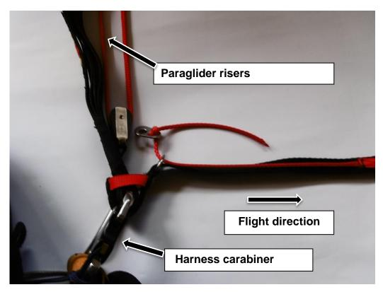
Illustration 4.1: Attachment to the harness left hand carabiner (without attachment of the pre-accelerator)
