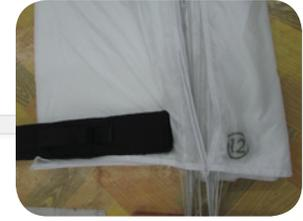
**10** 'S' fold the left hand side, this time on top of the existing folds to the width of the deployment bag.
