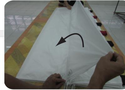
**8** The parachute should look as shown with the corner vent of panel 12\* in the middle and on top. The corner vent of panel 1 should be in the middle underneath. At this stage, again double check the lines are free of twists and run cleanly either side of the apex lines all the way to the bridle.
