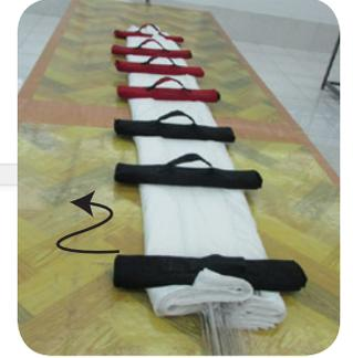
**11** Now arrange the lines keeping them neat and under tension. Use figure of 8 folds and elastic bands around the loops to arrange the lines neatly. The figure of 8s should be made to the same width as the deployment bag. Leave approximately 0.5m of line free at the end before the bridle.
